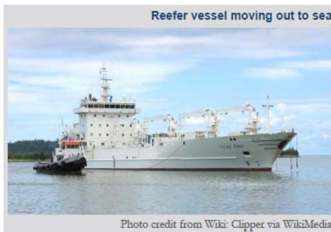
port structures, reefers are generally equipped with onboard cranes. These vessels tend to be small compared to container ships and bulk vessels.
